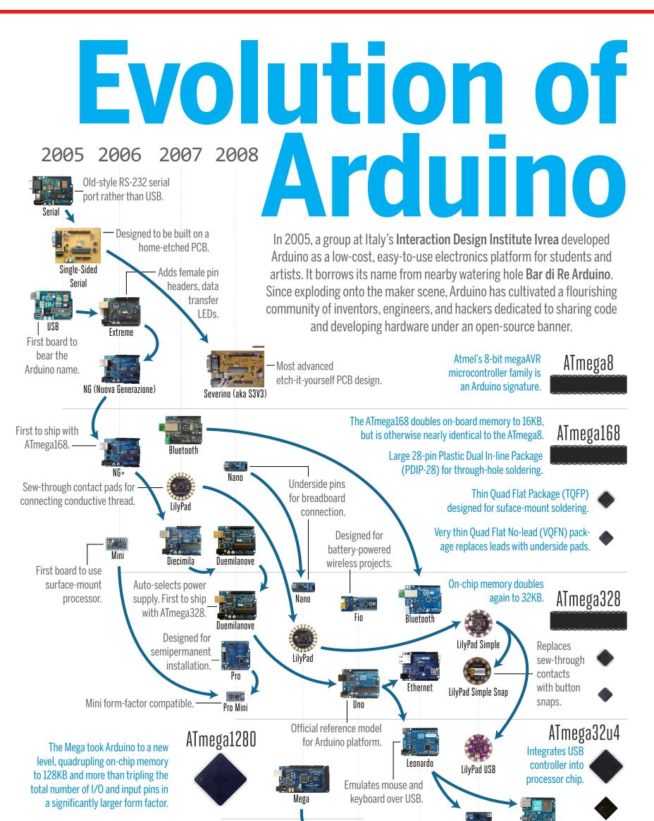
With the Mega2560, memory doubled again to 256KB. Though larger, the new form factor remains pincompatible with the standard Arduino shield footprint.
